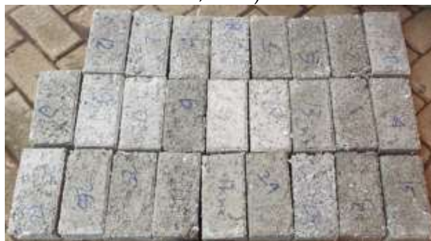
Figure 4. Printing and Curing Paving Block Using PET Plastic Mixture
